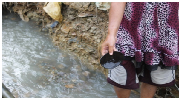
Plate 6. Bagol or coconut shell is used by a T'boli woman in stirring the water to facilitate catching of the gold particles
